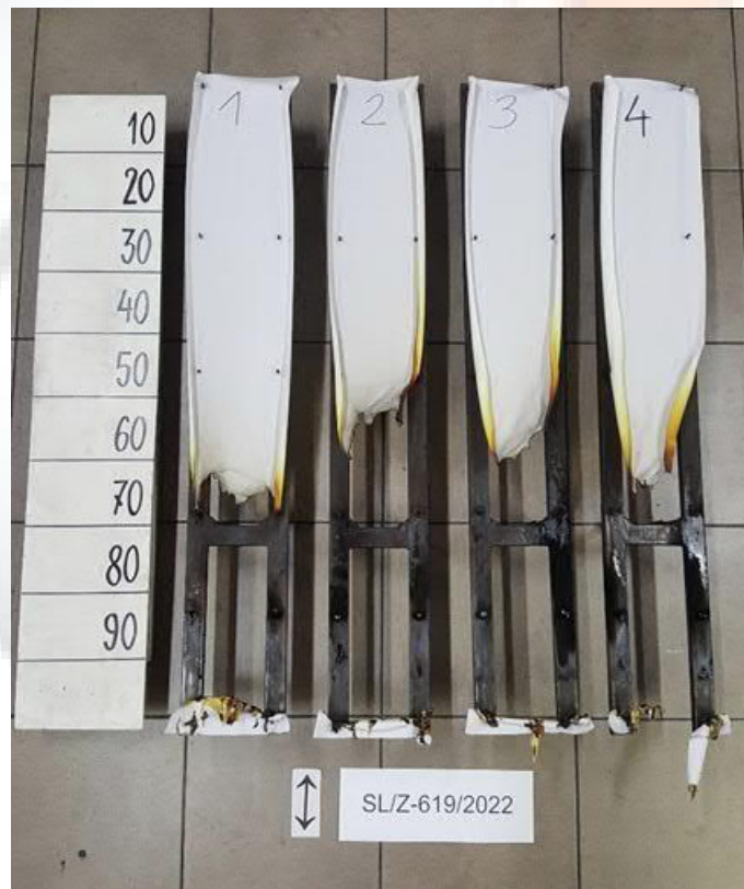
Figure 2. Appearance of the sample 1 after the test - length direction
