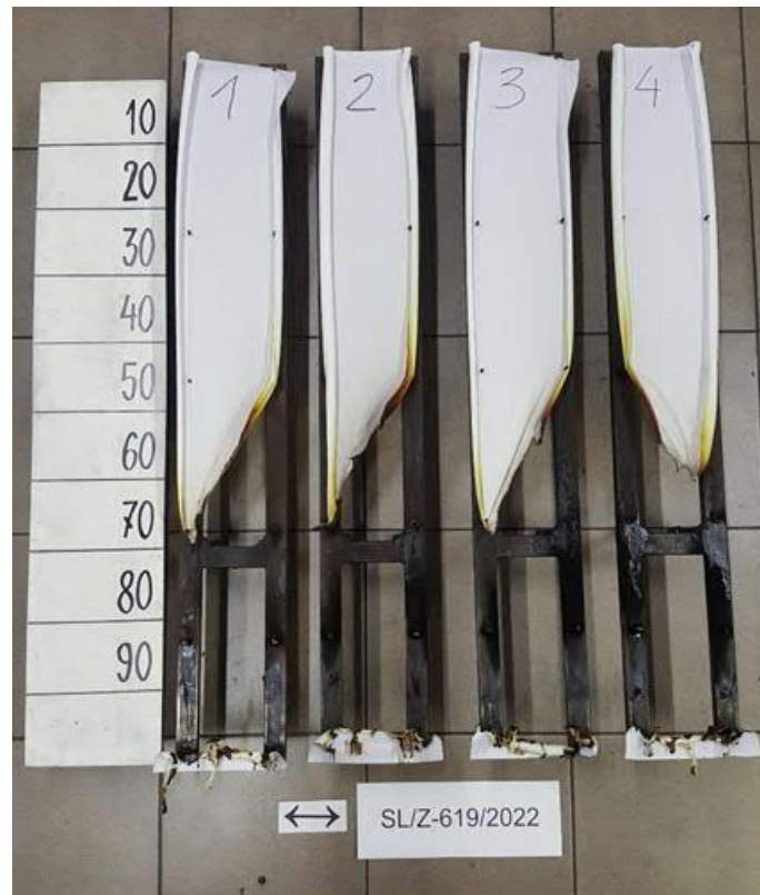
Figure 3. Appearance of the sample 2 after the test – cross direction
